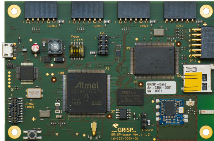
Figure 3.: GRiSP board - Image was taken from https://www.kickstarter.com/projects/peerstritzinger/grisp-2
